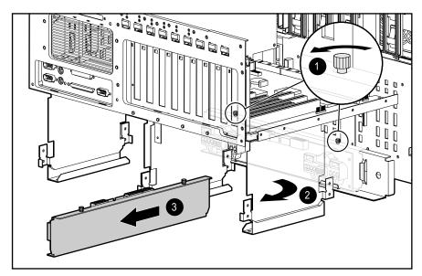
Figure 2-36. Removing the power backplane board
